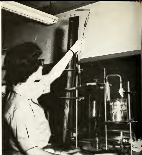
FLIP CLOSES STOPCOCK TO READ P. OF BENZENE.
