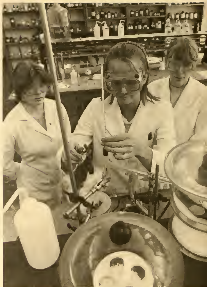
Chemistry students set up vacuum distillation apparatus.
